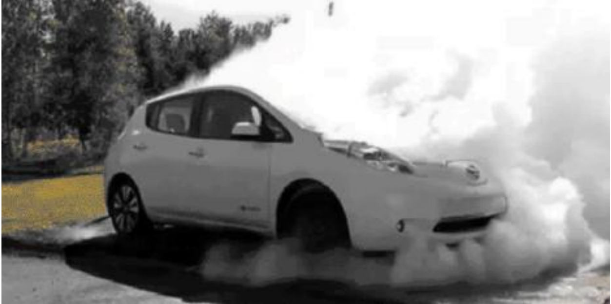
Figure 6 - EV in Thermal Runaway
