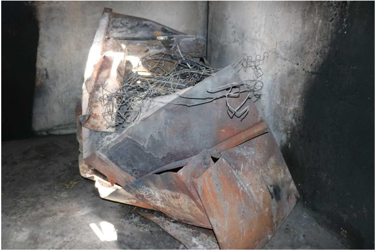
Burn Crib with metal parts of recliner base on top
