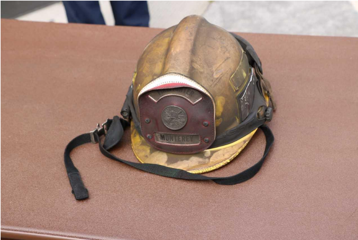
Helmet showing damage to Shield
