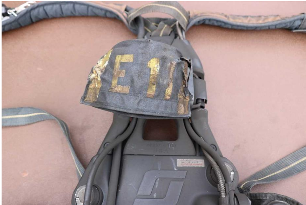
SCBA showing damage to Pack
