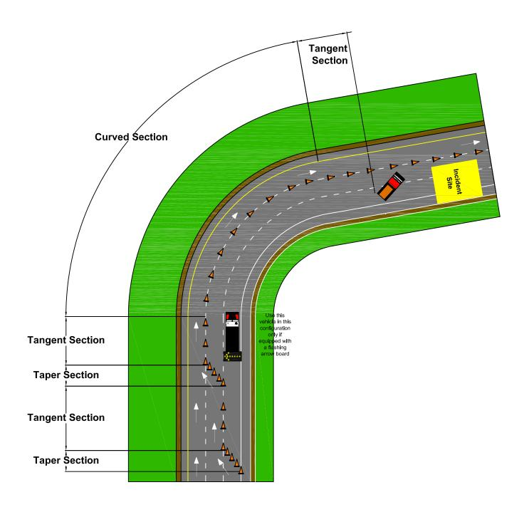
Fig. 14.2 - Tangents and Tapers in Curved Sections
