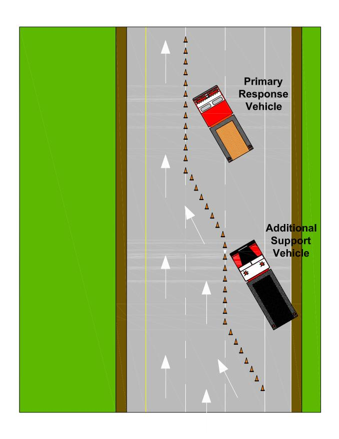
Fig. 10.1 - Use of Additional Support Vehicle
