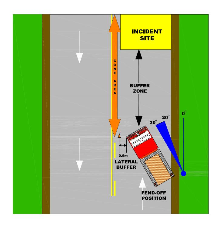
Figure 9.1 - Apparatus Staging
