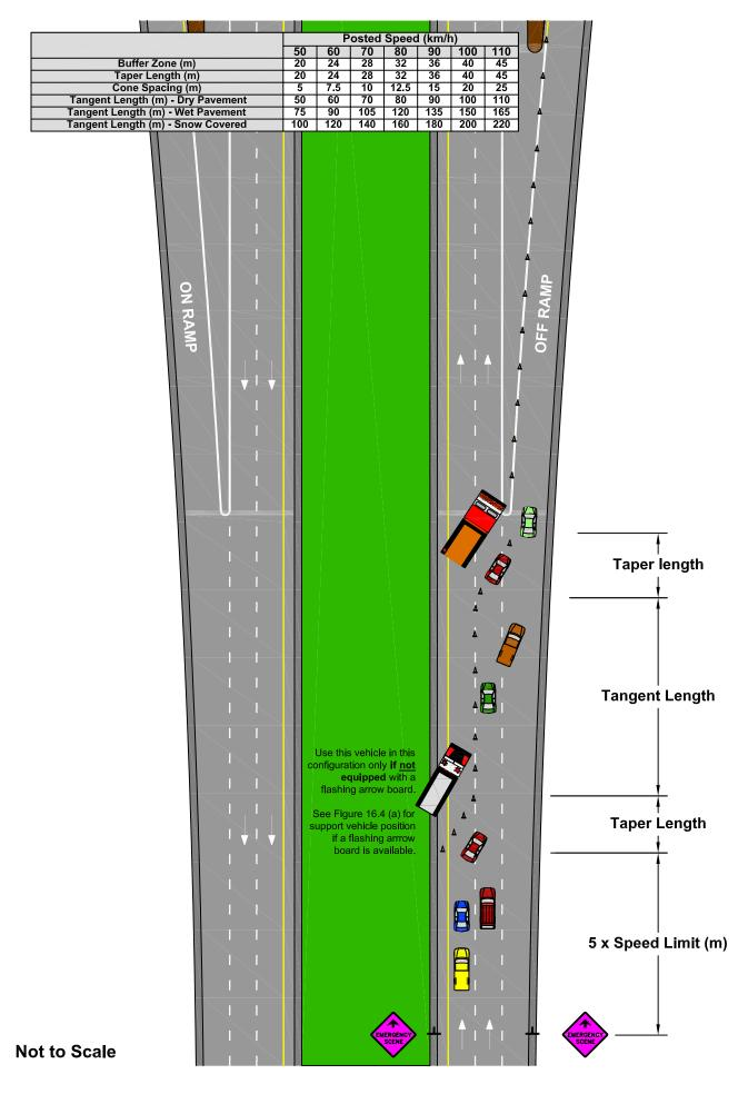
Fig. 16.6 - Controlled Access Highway - Detour
