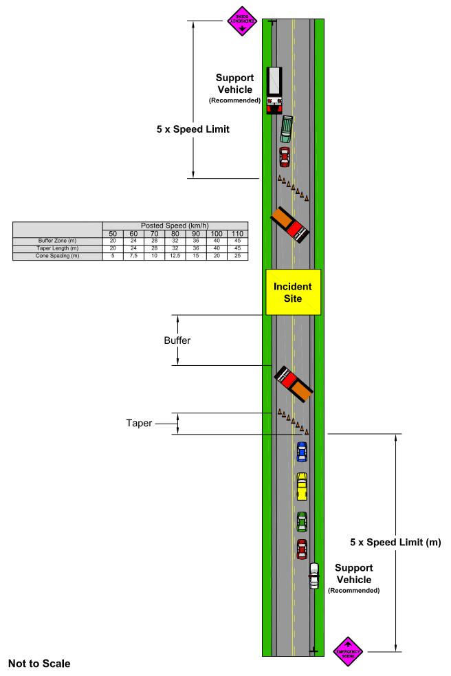
Fig 16.1 - Two Lane Two, Way Highway - Road Closed
