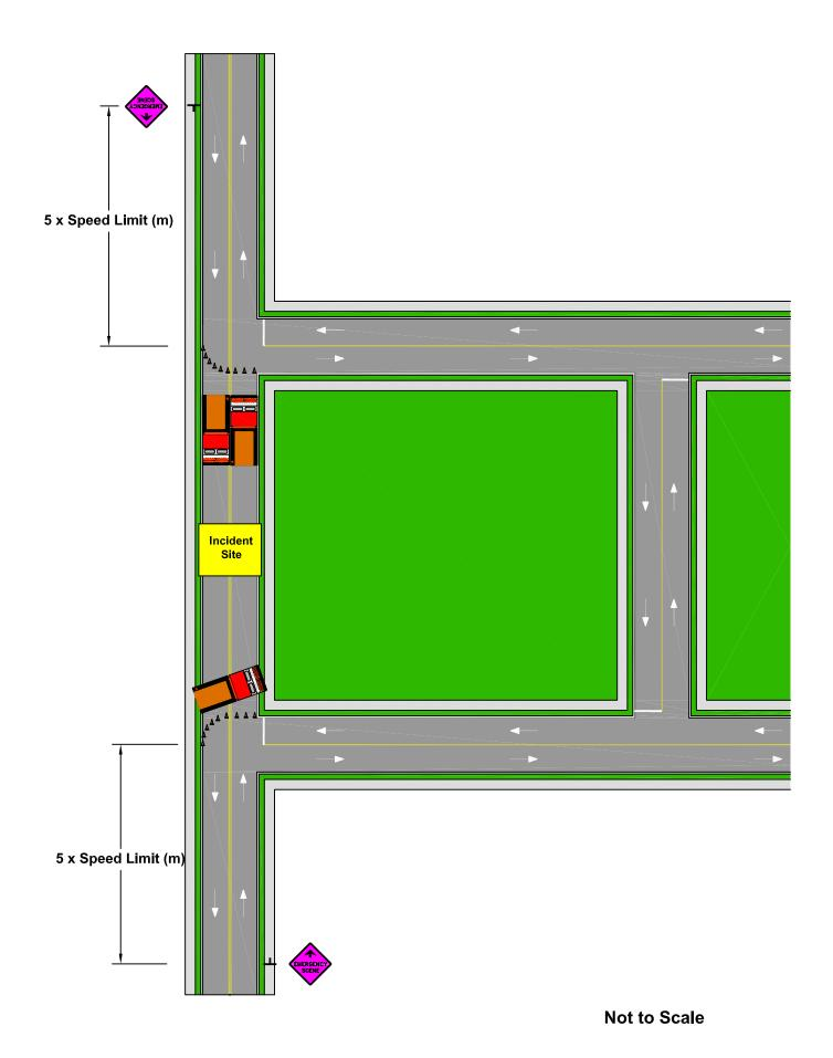
Fig. 16.5 - Two Lane Two Way Highway - Detour
