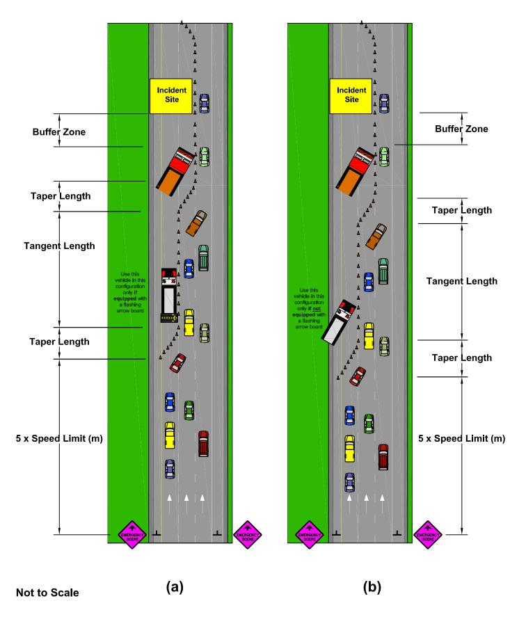
Fig. 16.4 - Multi-Lane Divided Highway - Two Lanes Closed
