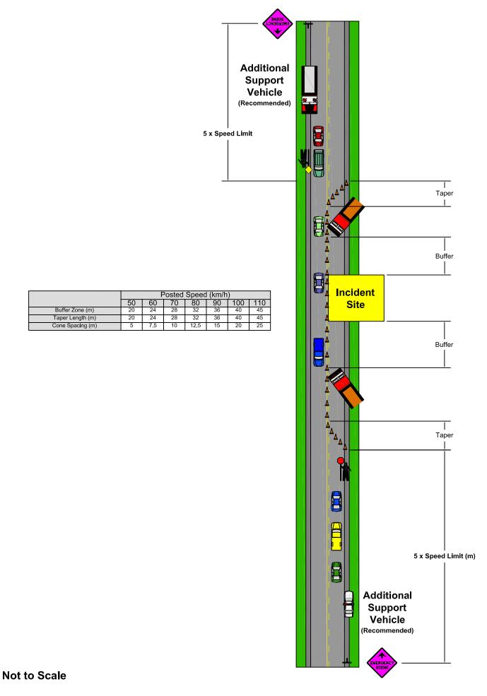
Fig 16.2 - Two Lane Two, Way Highway - One lane Closed
