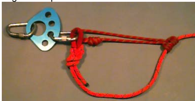
Figure 15 – Using a soft interface at the anchor.
