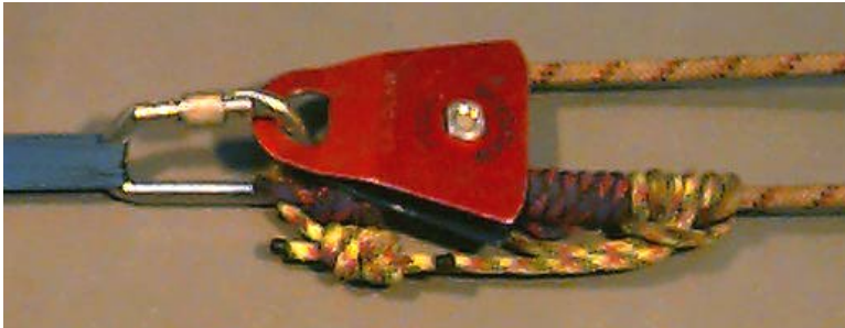
Figure 8 – Prusik minding pulley with fitted Prusik loops
