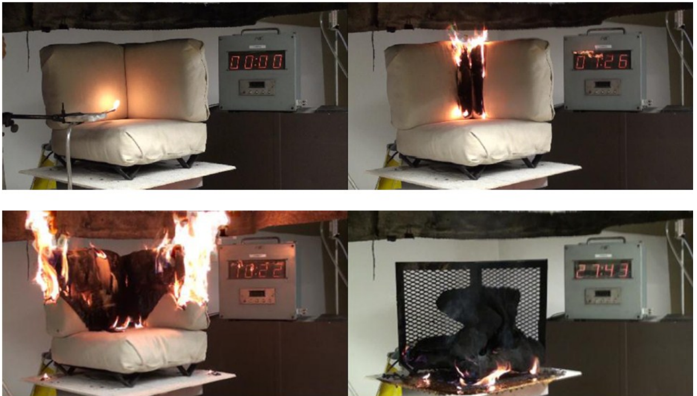
Upholstered chair with polyester wrap covered Cal TB 117 compliant fire retardant treated polyurethane foam cushions (20 s ignition flame exposure at the center of the seat-back cushions)
