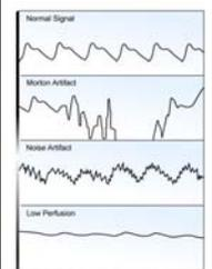
The effect of artifact on a pulsatile signal from an oximetry sensor
