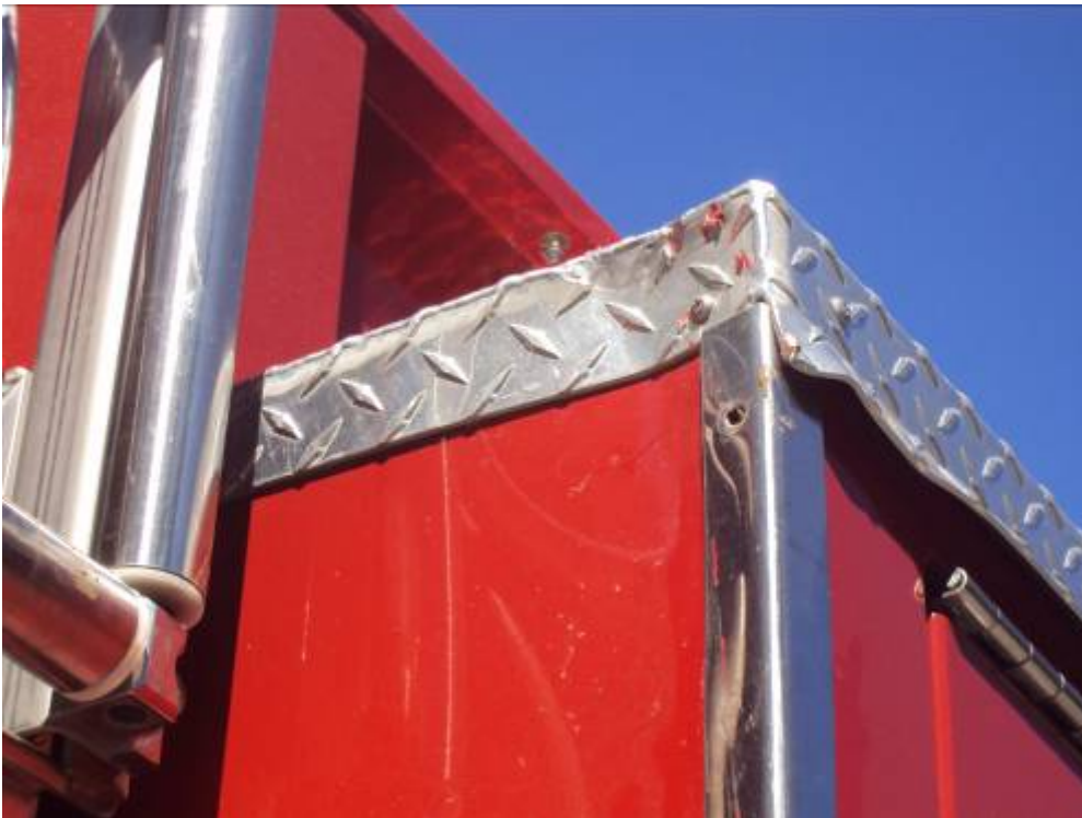
Damage to Engine 1169 – Driver's side compartment.
